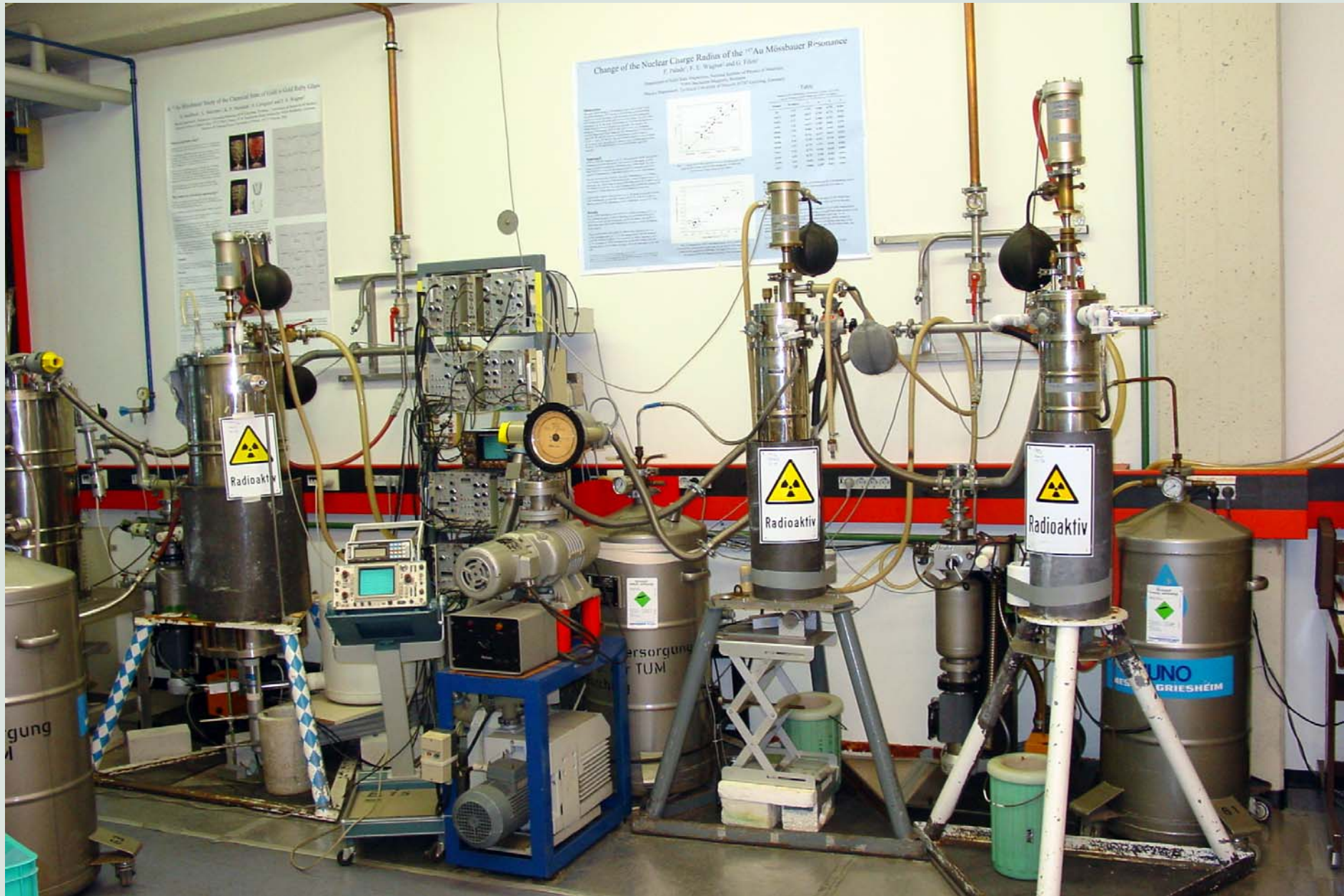
Measurements at liquid helium temperature: Source and absorber are at 4.2K, the counter is at RT.
