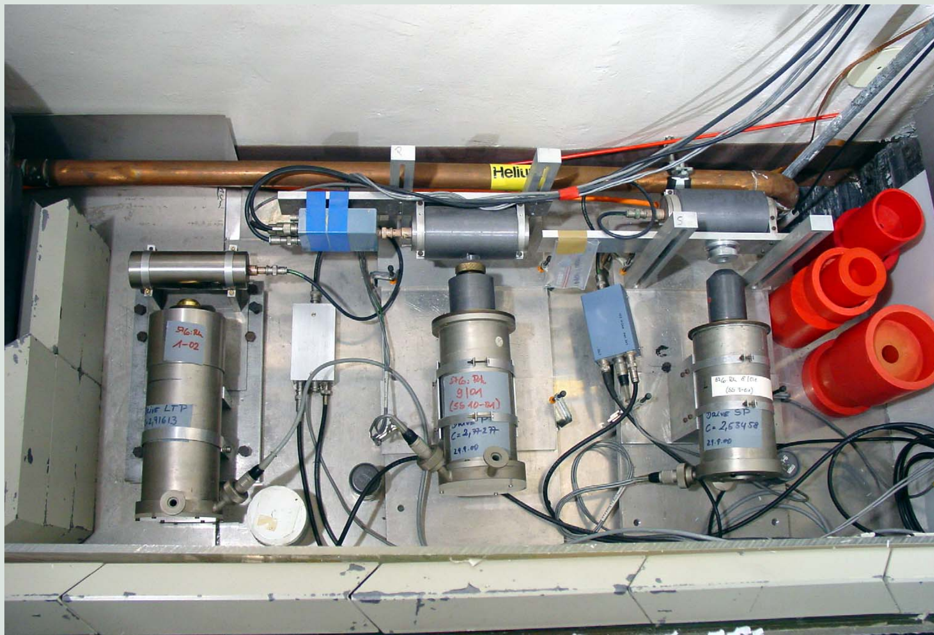
The ^{57}\text{Co} in Rh sources are mounted on the velocity drives. The counters are in back.
